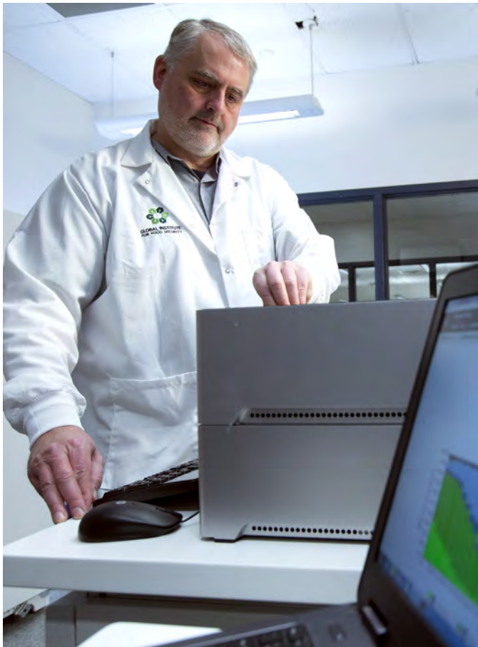
Dr. Andrew Sharpe with the PromethION, which is capable of completing DNA and RNA sequencing on a large scale at great speeds.
